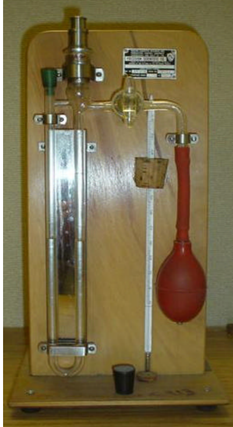
Figure 2.3 Air Permeability Apparatus (Blaine)
